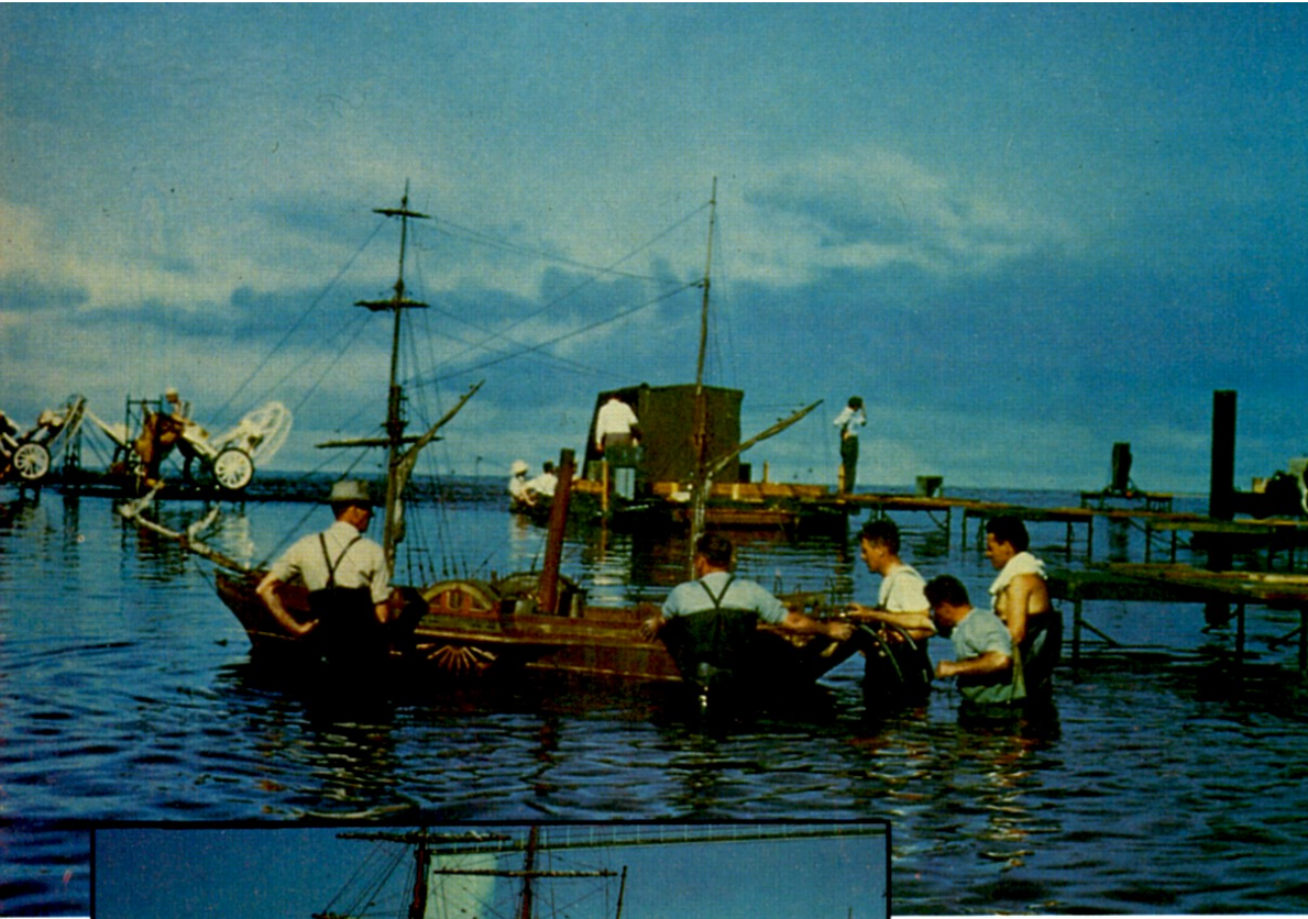
An effects crew rigs the model of the nitrate ship at Fox's Sersen tank. The free-floating model was designed to be pulled through the water by cables. Inset: The Abraham Lincoln and nitrate ship miniatures in their storage carriers.
